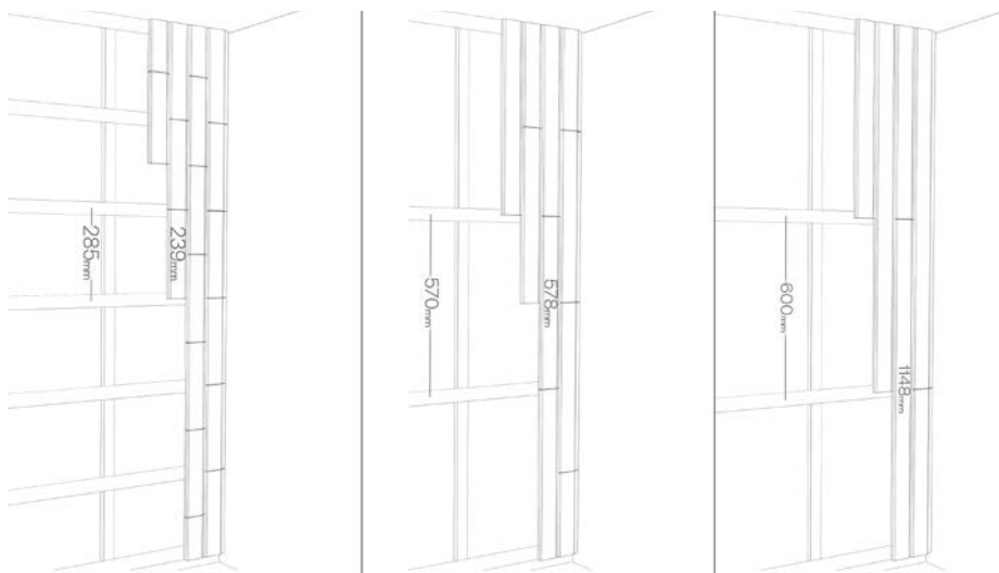
Tiles by Thermory panels vertical installation
